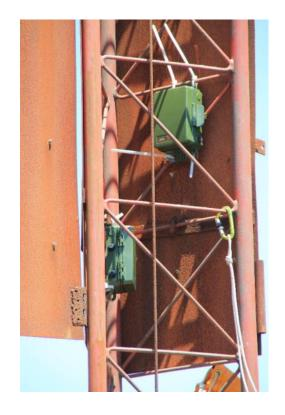
Photograph 7.15 - Automatic detectors installed on the meteorological mast
